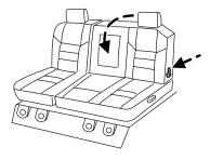
To flip the seat cushion up, pull up on the lever located on the side of the seat cushion to rotate the cushion up until it locks into a vertical storage position, gaining access to the grocery hook located on the underside of the driver-side seat cushion. The maximum load is 25 lb. (11 kg).
